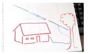
The three elements are connected, not separate as shown in the diagram. Coax goes to the first one as in a regular dipole. Second section is open wire line with a short in the middle (look closely) and it Does Not Radiate. High impedance at end of open wire matches and feeds end of 3<sup>rd</sup> half wave. The 2 half waves on each end radiate in phase and combine for 3dB gain broadside to antenna.
