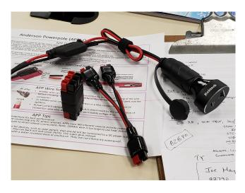
The connectors are rated for 10,000 cycles in and out, but if you unplug them 'hot' the rating drops to 250 cycles. Turn your stuff off before pulling the plug apart.
