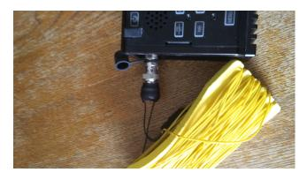
For quick setup Don made a 49:1 ratio balun to feed an End Fed wire that works 40 thru 10M. It's wound on a T47 core no larger than a dime so it won't take much more than the 5W output of the radio, but does make a pocket size package that will do wonders.
