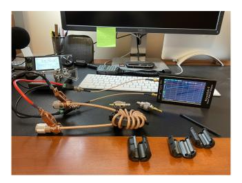
Remember this program by Gary JOK using his VNA to measure effective reactance of a coil used as part of an end fed antenna?
