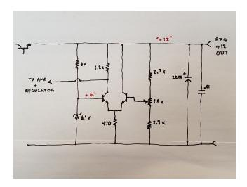
ZQG drew a schematic of 2 transistors in the classic differential amplifier layout often used in regulated power supplies with the Base of 1 going to the volt adjusting pot, and the other Base hooked to a 6.1 V Zener voltage reference diode. His question, "What happens to Base 1 when you turn the pot to increase output from, like, 12V up to 13.8 V?
