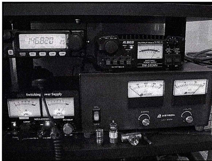
Left to Right excluding FT-2800 ALINCO 32 Amp switcher MFJ 4225 25A switcher ASTRON VS-35M
