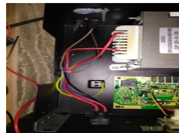
Figure 8: Power Switch and Resettable Fuse
